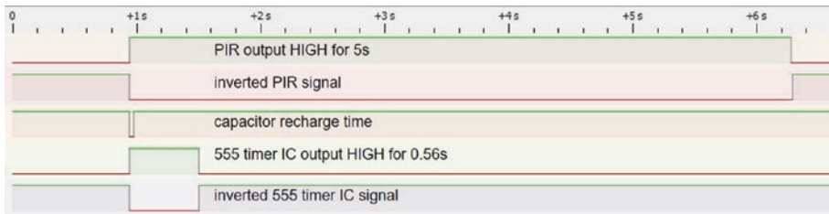
Figure 17-25. PIR sensor and MP3 player signal sequence
